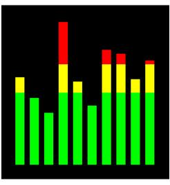
'min' and 'max' specify the range of values for the bar and, if specified, 'c1' to 'c4' and 'ta' to 'tc' specify the colours and thresholds for the analogue bar image. Note that unlike the circular bar gauge a "ghost image" of the colours is not shown in the background.
