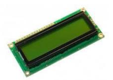
The following shows a typical usage where d4 to d7 are connected to pins GP2 to GP4 on the WebMite, rs is connected to pin GP6 and en to pin GP7.
