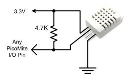
To get the temperature or humidity you use the HUMID command with three arguments as follows: DEVICE HUMID pin, tVar, hVar [,DHT11]
