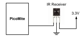
Vishay TSOP4838, Jaycar ZD1952 and Altronics Z1611A. Note that the I/O pins on the PicoMite are only 3.3V tolerant and so the receiver must be powered by a maximum of 3.3V.
