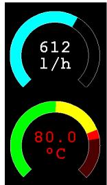
When colours and thresholds are specified the background of the gauge will be drawn with a dull version of the gauge colour at that level ("ghost colouring") so that the user can appreciate how close to the various thresholds the actual value is. Also the digital value displayed in the centre will also change to the colour specified by the
