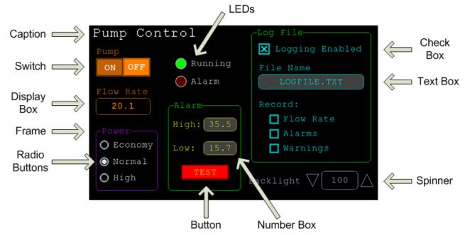
Each control has a reference number called '#ref' in the description of the control. This can be any number between 1 and the upper limit set by the OPTION CONTROL command. This reference number is used to identify a control. For example, a check box can be created with a reference number of #10:
