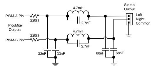
This circuit is suitable for general use; however more sophisticated designs can be used to improve the frequency response and reject more of the carrier frequency.
