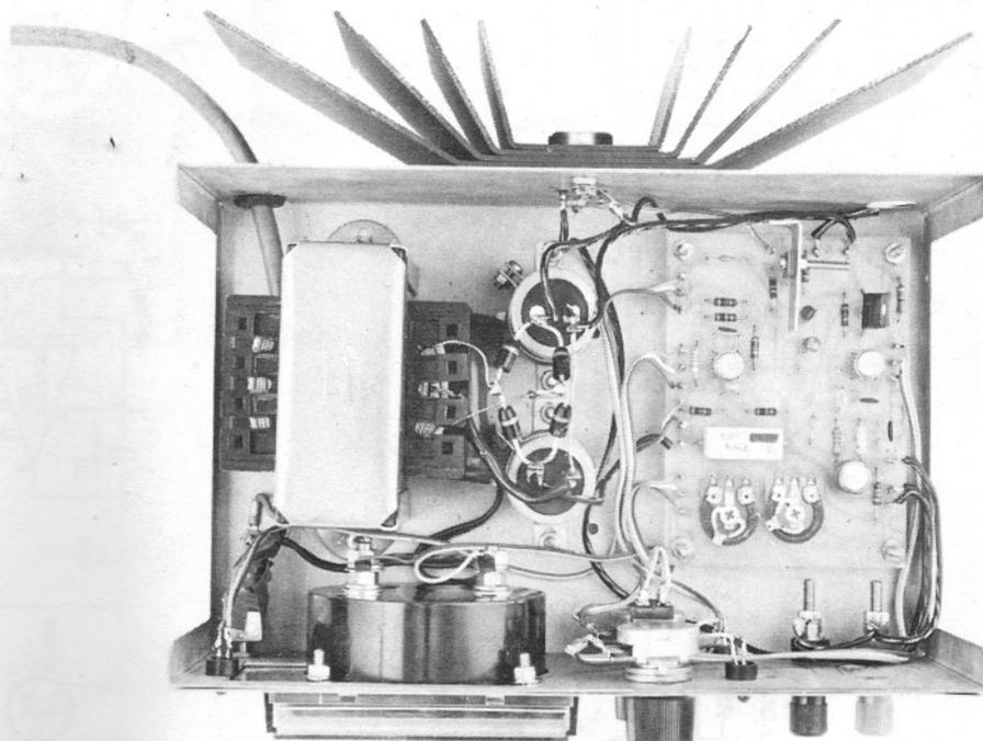
*Inside view of the completed 40 volt power supply. Note how the heatsink is mounted to the rear of the unit.*
