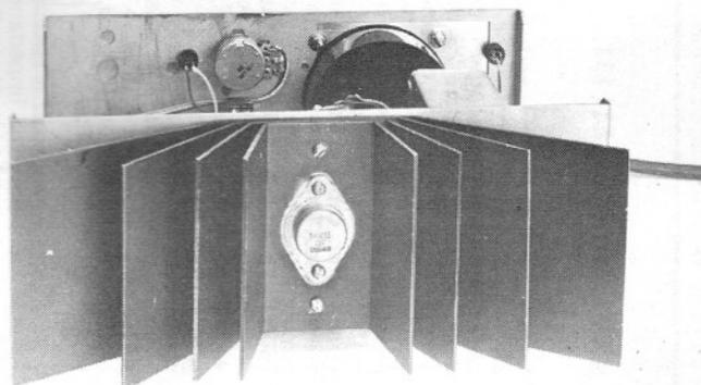
*Rear view of the heatsink showing how it and the transistor are mounted.*
