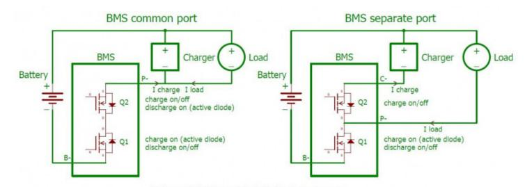
Discharge Mosfet Q1 is switched off when battery is empty Charge Mosfet O2 is switched off when battery is full
