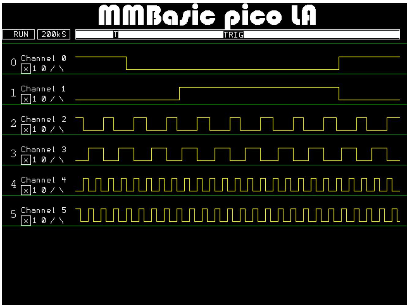
Above is just an example of various input signals to GP0...GP5 of the analyzer. As you will experience, the screen is constantly updating, showing you the live behaviour of the input signals. In case you want to study the signals you can stop the analyzer by using the PicoMiteVGA keyboard.
