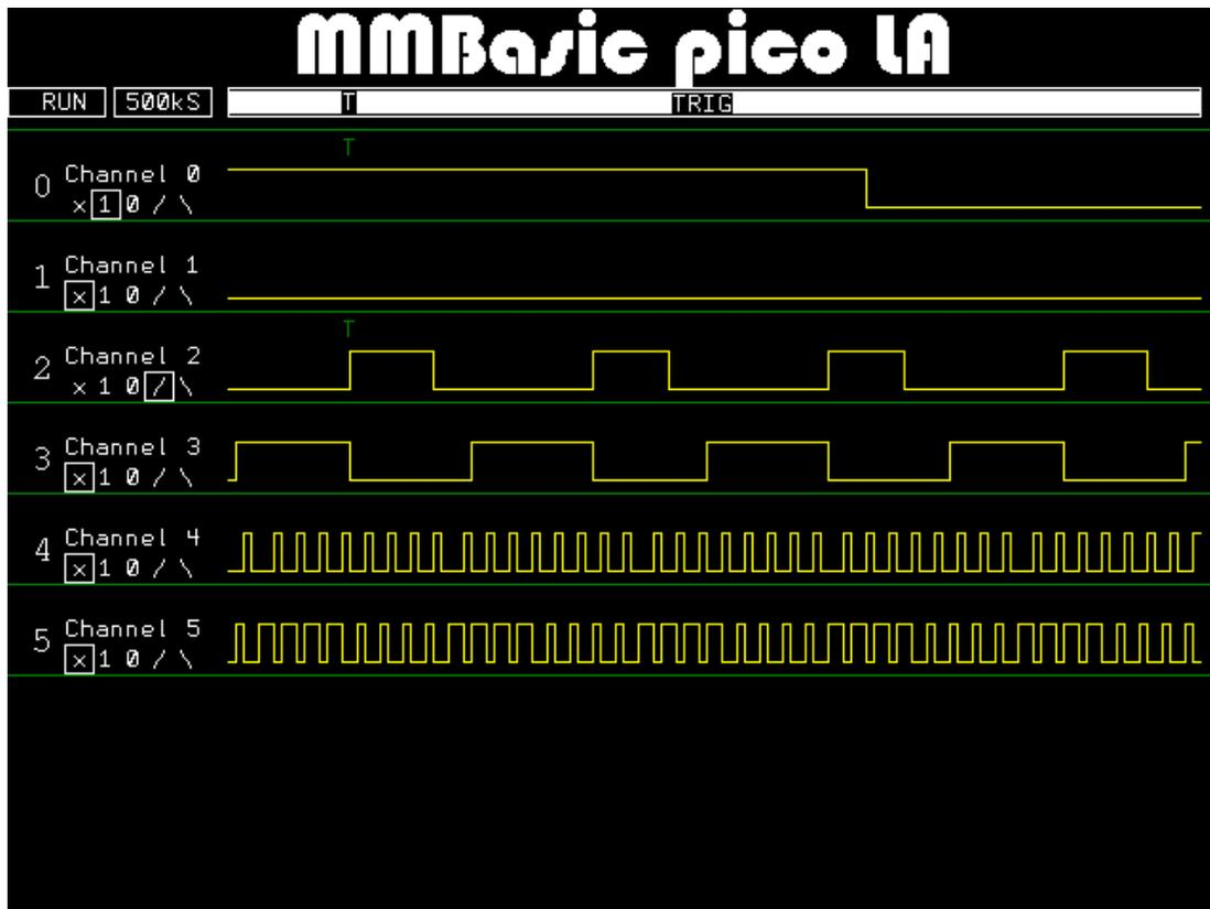
When setting up a trigger condition, you **ARM** the logic analyzer. Once the event has occurred, the logic analyzer is **TRIG**gered.
