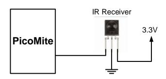
Vishay TSOP4838, Jaycar ZD1952 and Altronics Z1611A. Note that the I/O pins on the Raspberry Pi Pico are only 3.3V tolerant and so the receiver must be powered by a maximum of 3.3V. The Raspberry Pi Pico 2 is different and can withstand 5V.
