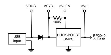
For embedded controller applications generally an external power source (other than USB) is required and this can be connected to VSYS via a Schottky diode. This will allow the Raspberry Pi Pico to be powered by whichever supply is producing the highest voltage (USB or VSYS). The diodes will prevent feedback into the lower voltage supply.
