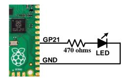
When you have saved and run this program you should be greeted by the LED flashing on and off. It is not a great program but it does illustrate how the PicoMite firmware can interface to the physical world via your programming.
