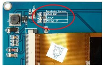
used to short the nearby pair of solder pads marked "1963-PWM". The brightness can then be set using the BACKLIGHT command via the SSD1963 controller (this is automatic, nothing needs to be configured).
