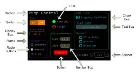
These functions make it easy to create a control panel to manage any control functions like a lathe, motor controller, heating system, small industrial process and so on.
