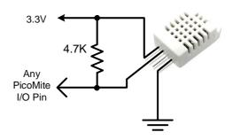
To get the temperature or humidity you use the HUMID command with three arguments as follows: HUMI D pi n, tVar, hVar [, DHT11]
