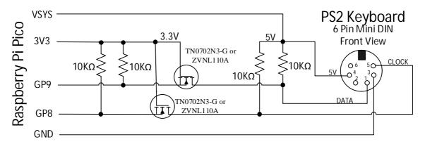
The recommended MOSFET is a TN0702N3-G or ZVNL110A however the commonly available 2N7000 has been tested and also works well.
